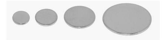
Magnetic metal specimen support discs are used on the AFM /SPM systems which employ a button magnet to hold the metal specimen disc. The metal specimen discs provided by NanoAndMore are made of a magnetic type 430 stainless steel with a nominal thickness of 0.90mm and a tolerance of +/- 0.08mm.
